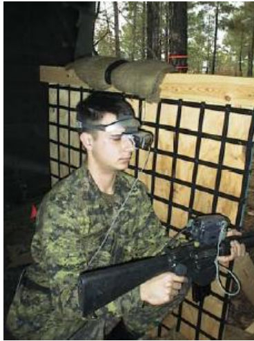
Figure 7 - Head mounted displays with weapon-mounted off-bore systems
