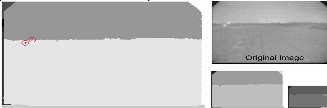
**Figure 8 - Region Segmentation of the Approximate Night Vision Intensified Image at Three Levels of Decomposition: Level 1 - left, Level 2 - middle and Level 3 - right (After: Chow, 2004)**
