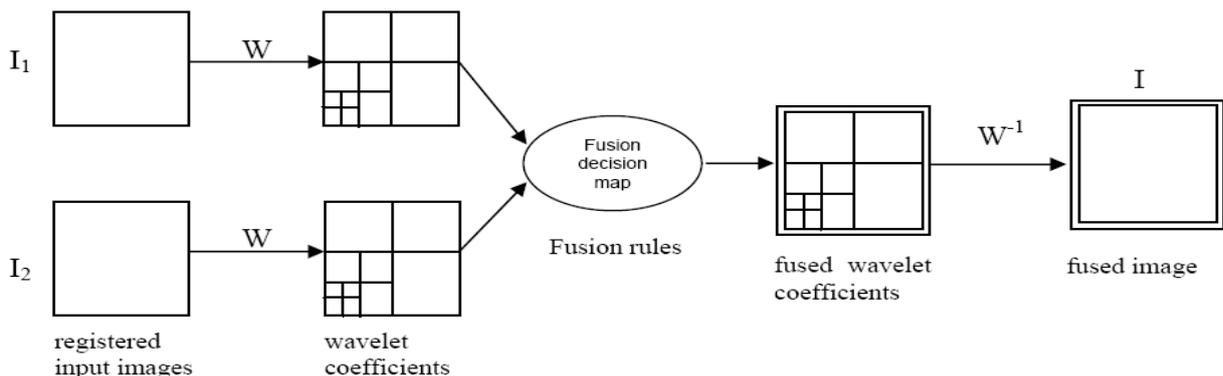
**Figure 6 - General framework for wavelet transforms fusion. (After Chow, 2004)**
