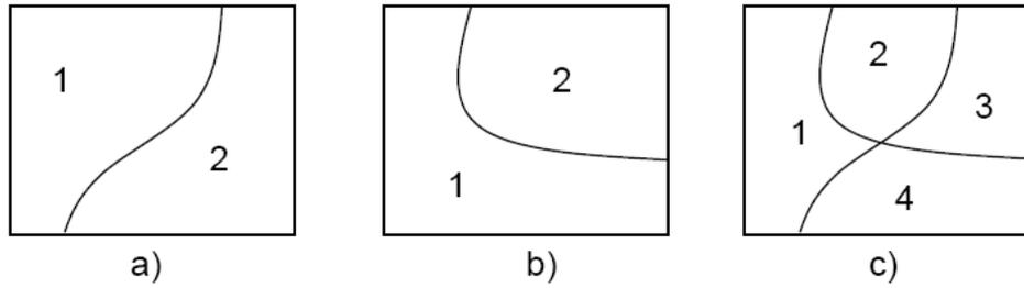
**Figure 10 - Region Segmentation: a) Region Representation of Image A; b) Region Representation of Image B and c) Joint Region Map, Indicating the Four Identified Regions. (From: Chow 2004)**
