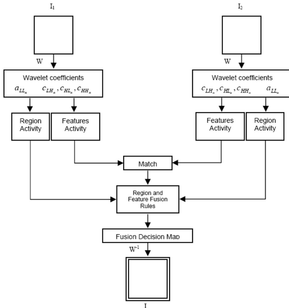
**Figure 11 - Framework for the Formation of the Fusion Decision Map for Region-based Fusion. (After: Chow, 2004)**
