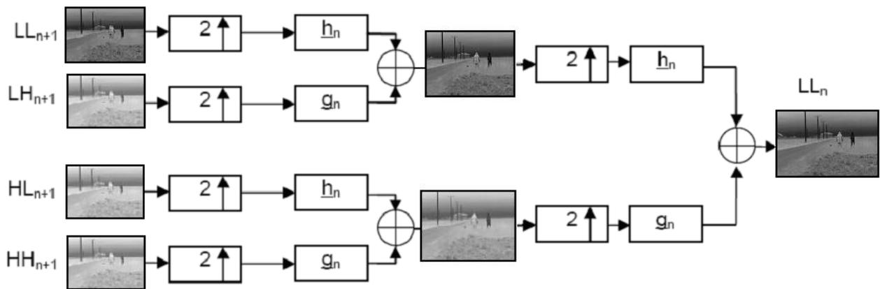
Figure 4 - Reconstruction Tree from 4 Subband Images Back to Recover the Original Image. (After: Chow 2004)
