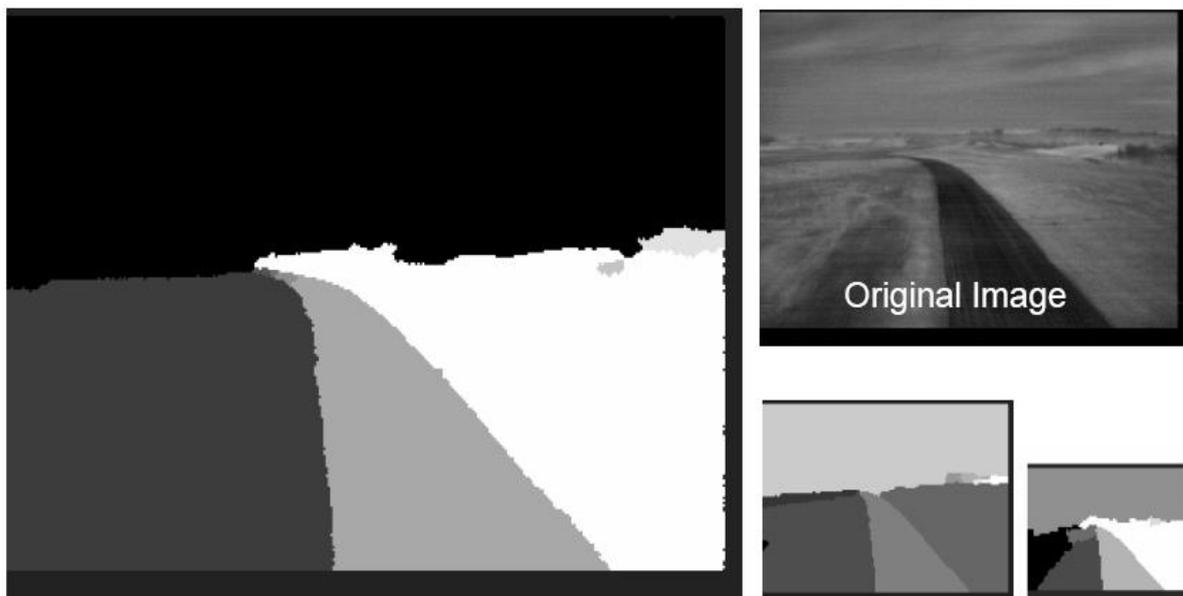
**Figure 9 - Region Segmentation of the Approximate Thermal IR Image at Three Levels of Decomposition: Level 1 - left, Level 2 - middle and Level 3 - right (After: Chow, 2004)**
