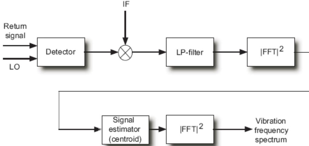
Figure 1. Block diagram of CW spectrogram processor.
