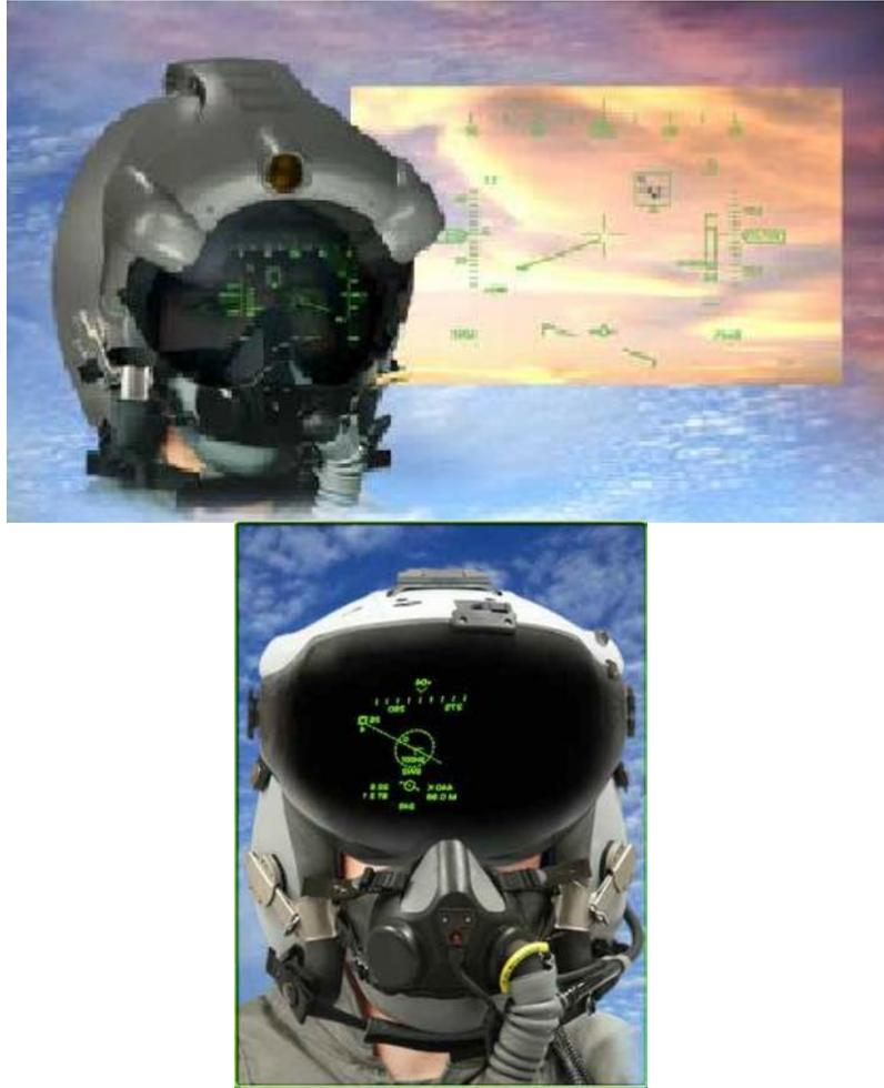
**Figure 9:** Examples of head-mounted projective display (HMPD)
